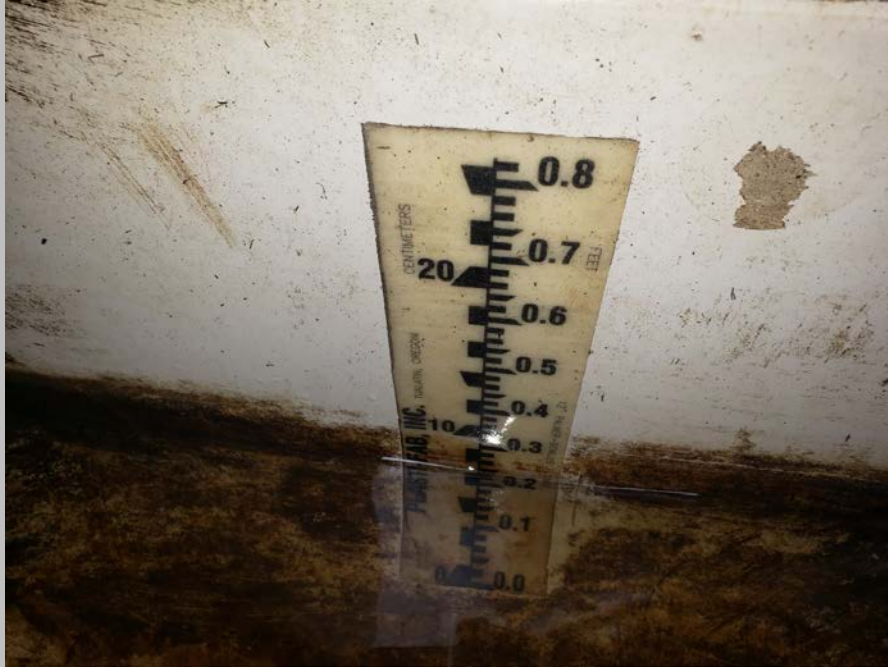
Stage on Flume = 0.24'
